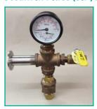
The Steam In Place (SIP) assembly allows you to turn a length of stainless steel sanitary pipe into effectively an autoclave. By applying low pressure steam at not greater than 20psi, an internal pipe temperature can be maintained in excess of 250°F (121°C) to achieve medical grade sterilization.
